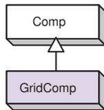
The triangle indicates an inheritance relationship. Inheritance means that a child class shares a set of characteristics (such as the same attributes or methods) with a parent class. The child can specialize and extend the behavior of the parent. This diagram shows a GridComp class that inherits from a more general Comp class.
