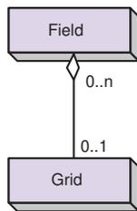
This simple diagram shows that a public class called Field is associated with another public class, called Grid. The aggregation relationship indicated by the unfilled diamond means that a Field contains a Grid, but that a Grid can be created and destroyed outside of a Field. The diagram multiplicities show that a Field can be associated with no Grid or with one Grid, but that a single Grid can be associated with any number of Fields.
