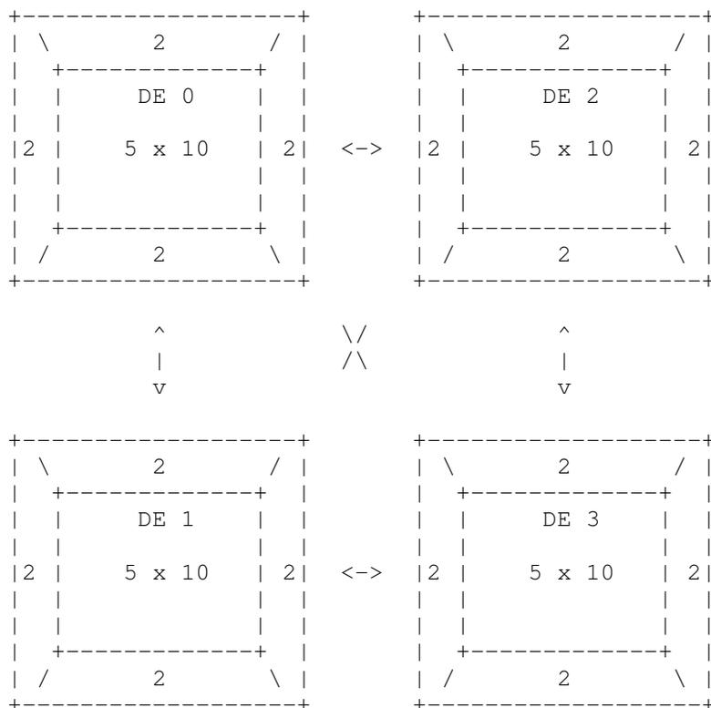
The exclusive region on each DE is of shape 5 x 10, while the total region on each DE is of shape (5+2+2) x (10+2+2) = 9 x 14. In a typical application the elements in the exclusive region are updated exclusively by the PET that owns the DE. In this example the exclusive elements on every DE are initialized to the value  $f(i, j)$  of the geometric function
