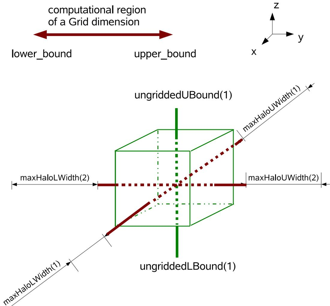
ESMF\_Field created from a 2D ESMF\_Grid (Red) and a 3D Intrinsic Fortran data array (Green). The ungridded bounds and halo widths are applied to corresponding dimensions.
