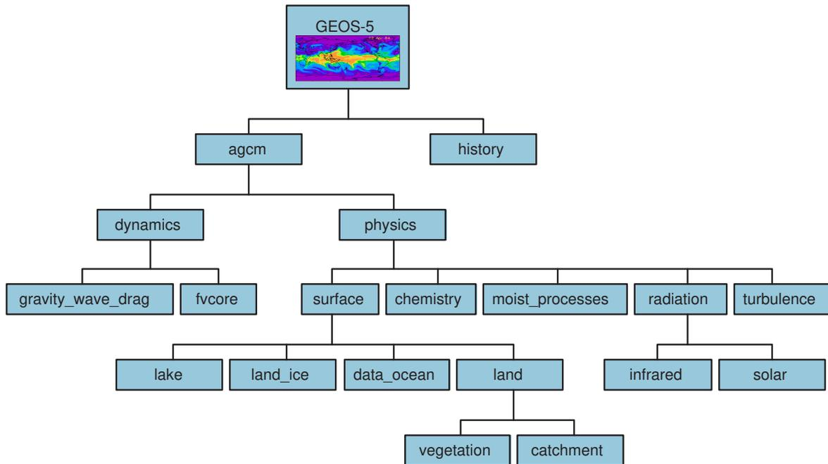
An ESMF coupled application typically involves a parent Gridded Component, two or more child Gridded Components and one or more Coupler Components.
